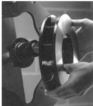
Remove the disc without removing or disassembling the brake.
